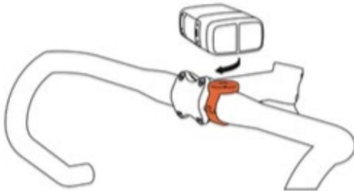
2. With your Fly12 facing forward, and at a 45° angle, line up the quick release male component on the Fly12 with the female receptor on the handlebar mount. Place the Fly12 into the mount and make a 1/8<sup>th</sup> turn until the device clicks into a forward-facing position. The distinctive 'click' sound confirms the unit has been locked in place.
